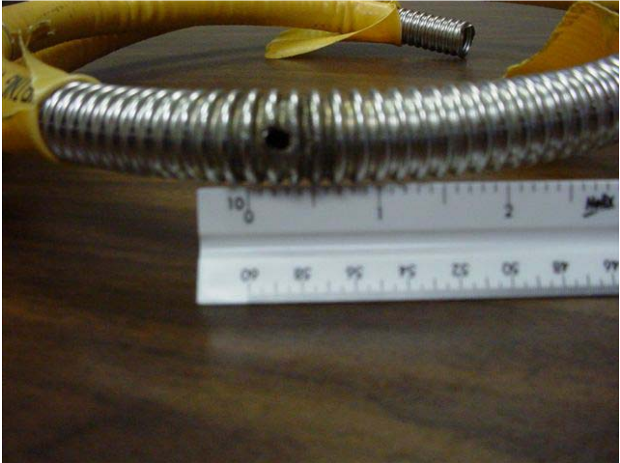
Typical Lightning Damage to CSST
